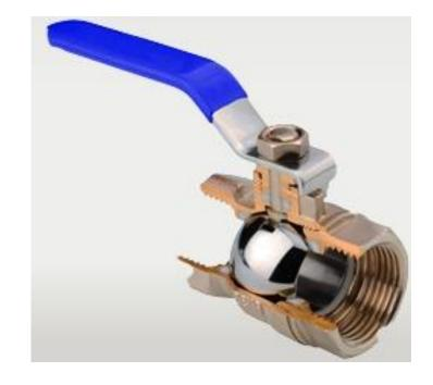
However, standard ball valves do not offer the fine control that may be necessary in throttling applications, but V ported ball variations are available for control purposes. The unrestricted bore in full bore ball valves make them ideal for hot tapping and pigging.
